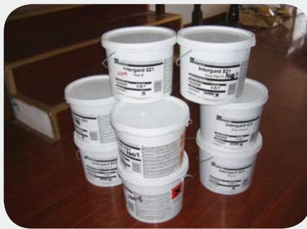
Epoxy filler for ICCP Di-electric shield
