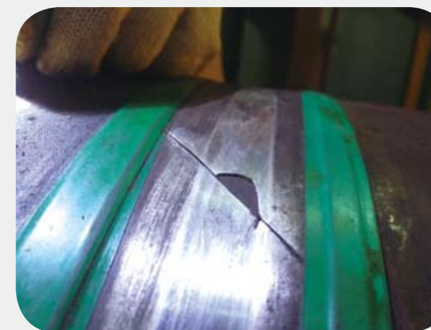
Faulty slip ring
