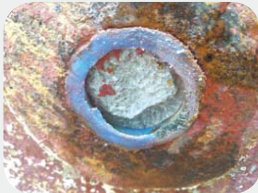
Ref. cell in poor condition
